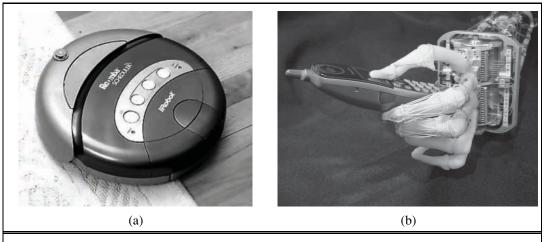
**Figure 25.30** (a) Roomba, the world's best-selling mobile robot, vacuums floors. Image courtesy of iRobot, © 2009. (b) Robotic hand modeled after human hand. Image courtesy of University of Washington and Carnegie Mellon University.
